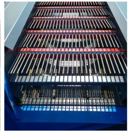
The Ultra Deck Deck screen is a compact screening unit, with features usually seen on larger machines.
