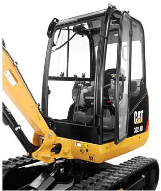
The Cat 302.4D cab is amongst the largest in the industry. The flat cab floor optimizes visibility and increases operator leg room. The ergonomic control layout provides a comfortable, highly productive workspace.
